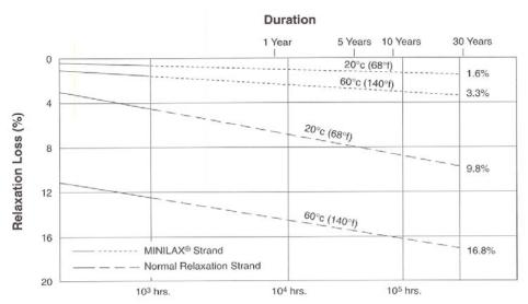
NOTE: Initial load is 70% of specified minimum breaking strength.
