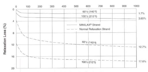
NOTE: Initial load is 70% of specified minimum breaking strength.
